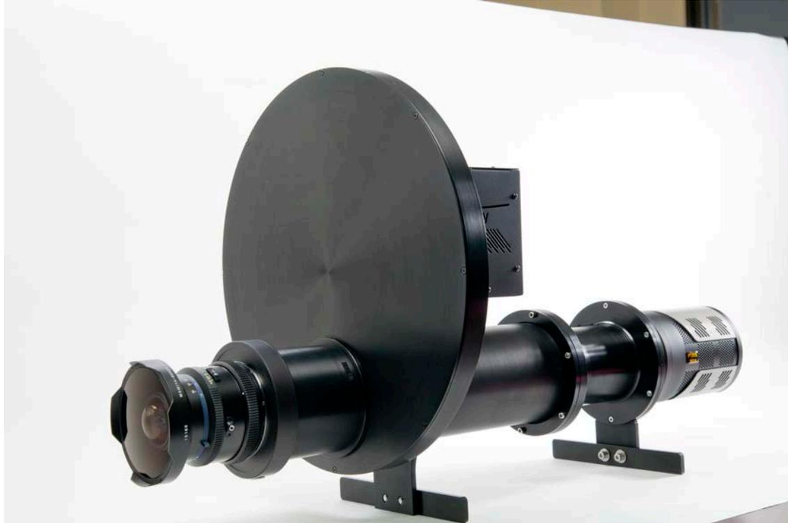
allsky lens is telecentrically imaged onto a 6-position filter-wheel (8-position also available) containing ~2-nm narrow-band interference filters. A single-filter-slot (no wheel) version is available as well.
