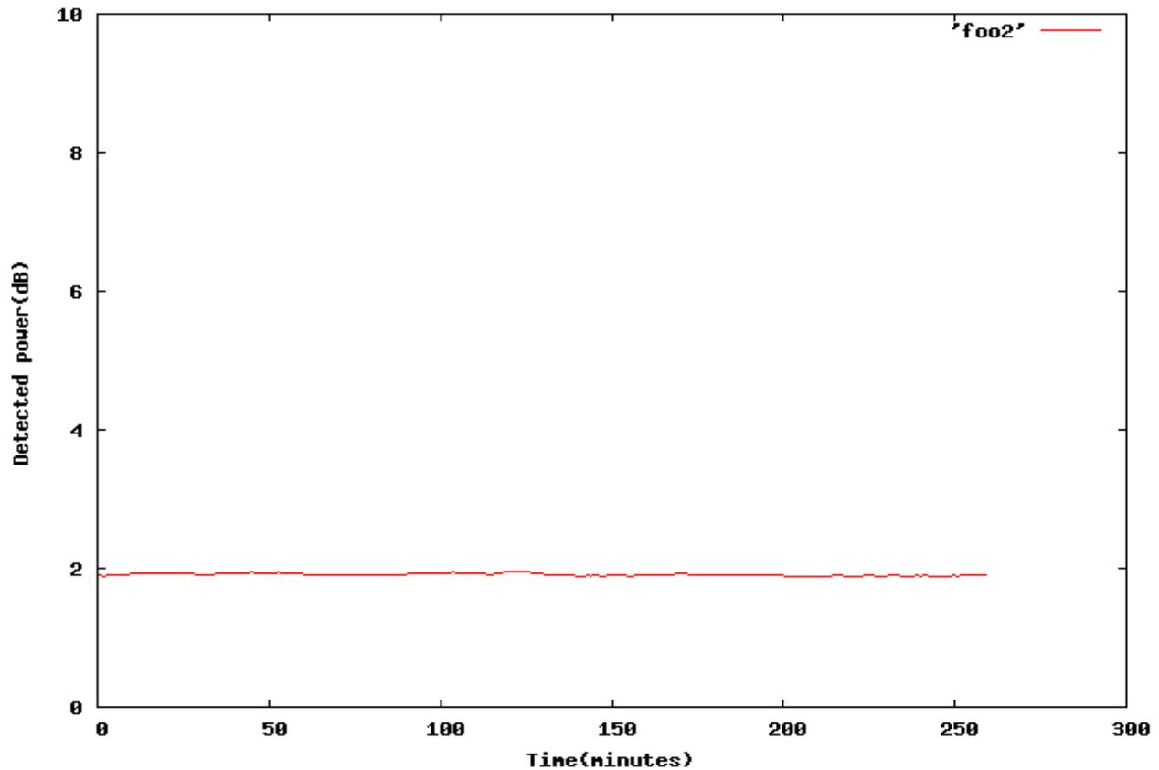
In field deployment, the front-end unit will be held to a constant 40C, and surrounded in foam insulation to reduce temperature variability, which improves both gain stability and stability of the reference termination used for switching.
