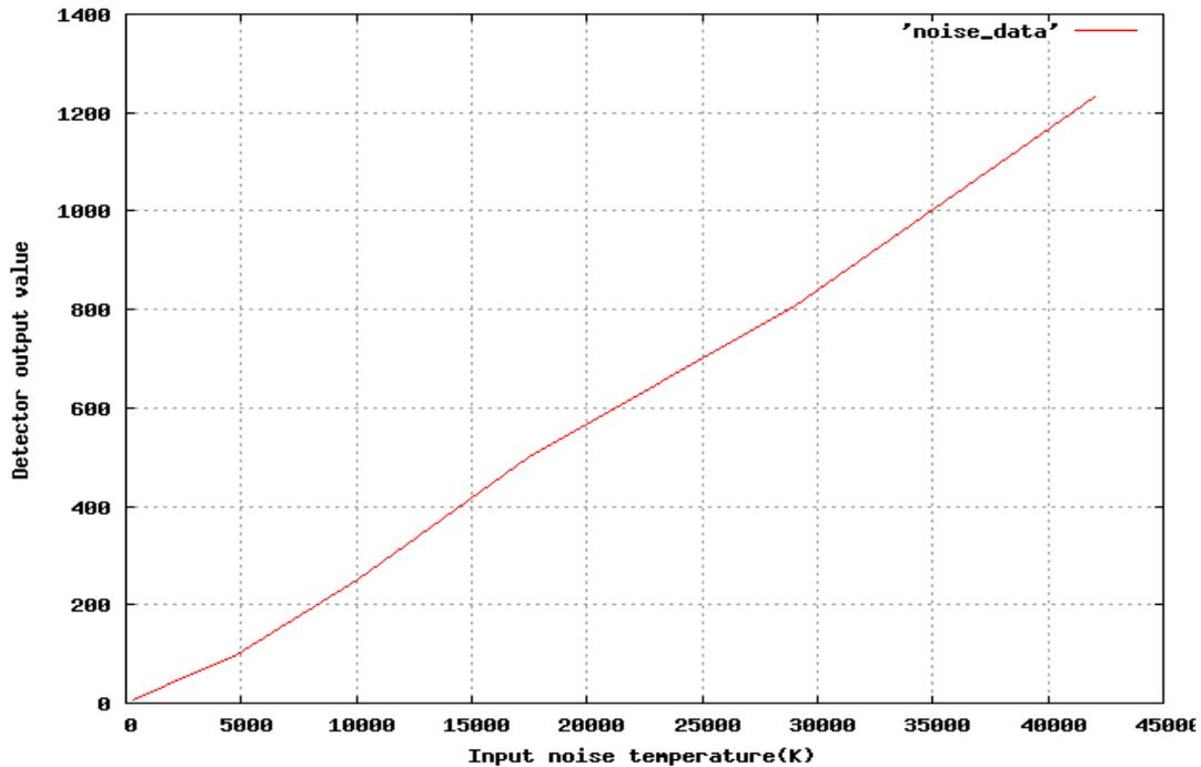
Above a plot of actual detector output values vs input noise temperature, for a variable noise source capable of producing noise outputs over the range of 290K to 42000K. Minor excursions from linearity are due largely to uncertainty in the calibration curve of the noise source.
