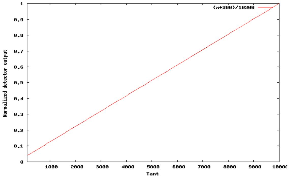
The smaller the value of  $T_{sys}$ , the closer to zero the detector output function intercepts the Y axis for zero input power.
