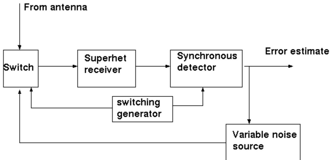
The measured-quantity in a Ryle-Vonberg receiver is the so-called *error estimate*, which acts as a kind of proxy for the incoming noise power. A *Ryle-Vonberg* receiver strives to balance the noise power offered by the noise source against the noise power coming from the antenna, and the magnitude of the *error estimate* signal is directly related to the magnitude of the incoming sky noise.
