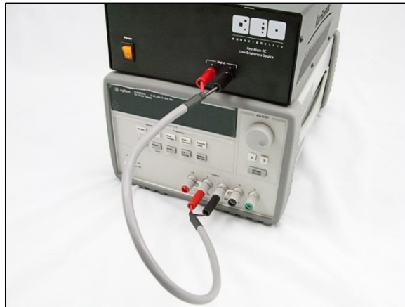
Figure 5: Agilent Banana Jumper Cable Connection
