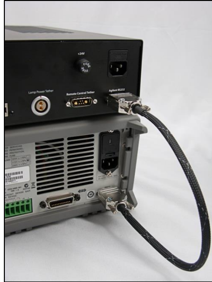
Figure 4: Agilent RS232 Cable Connection
