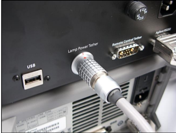
Figure 6: Lamp Power Tether Cable Connection 1
