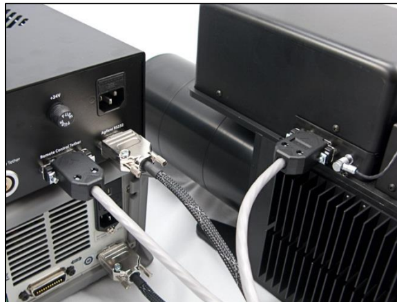
Figure 8: Remote Control Tether Cable Connection
