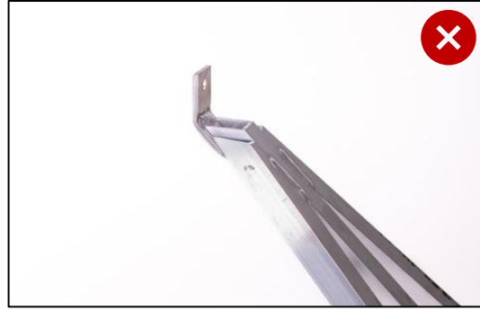
Figure 17: Incorrect antenna element orientation
