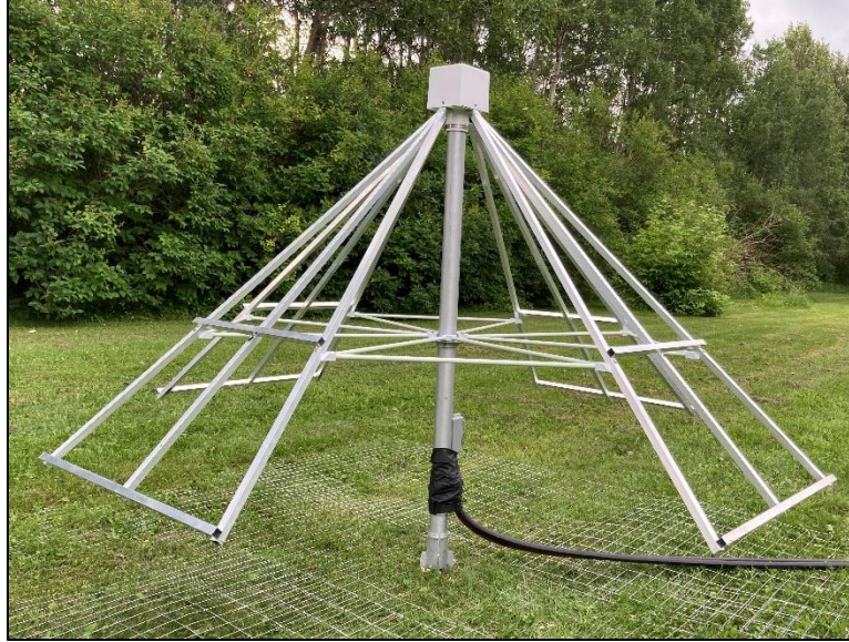
Figure 3: Riometer antenna deployed in the field with wire-mesh ground plane
